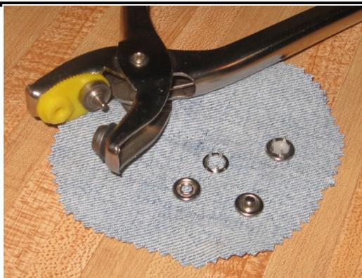
These pliers have a round metal holder on one side, and a yellow plastic (moveable) piece that has a round plastic holder and a metal punch. The metal punch is for grommets and eyelets. Make sure this is turned away to the back for snaps.
